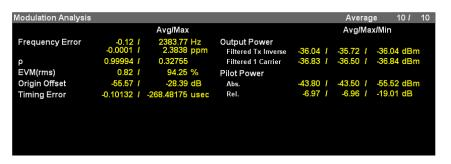
Figure 3.8-1 Modulation Analysis window
